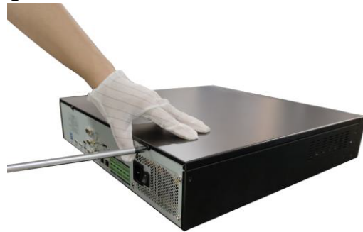
Figure 1-15 Install the cover and screws
