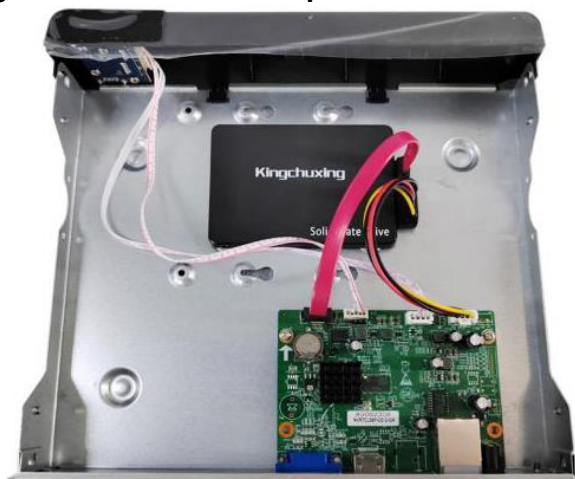
Figure 1-18 Connect the power and data cables
