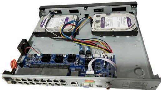
Figure 1-10 Connect the power and data cables
