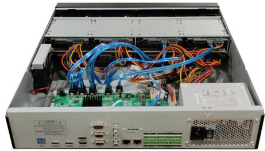
Figure 1-13 Connect the power and data cables
