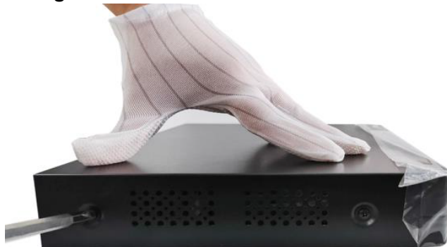
Figure 1-19 Install the cover and screws
