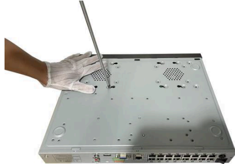
Figure 1-9 Install the HDD
