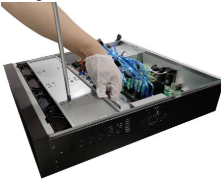
Figure 1-14 Install the HDD
